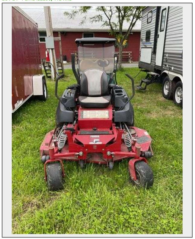
**Description**Ferris is2200 with 412 hours, 60 inch cut, vanguard big bore 32hp motor, runs and drives
